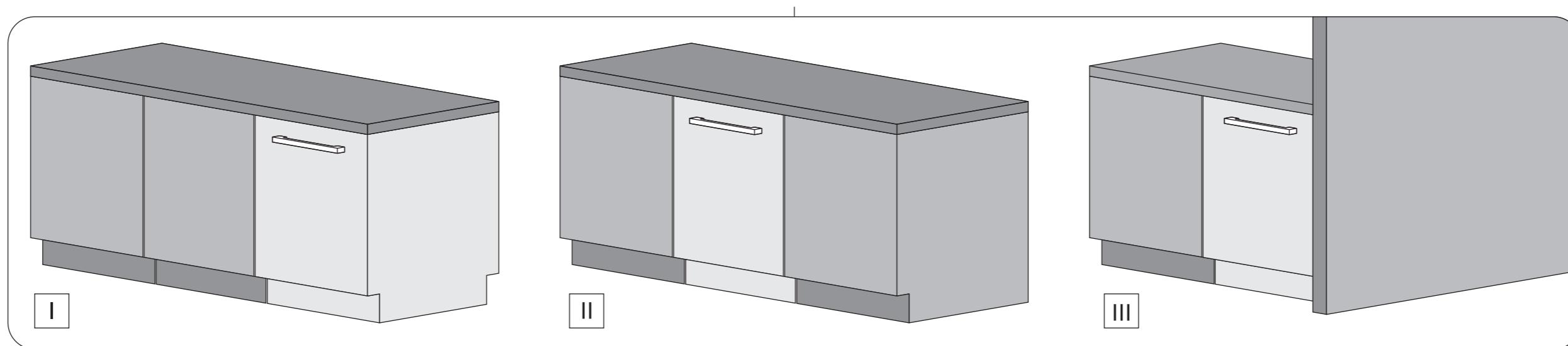
\*Align the center line with the center line of the wooden door
